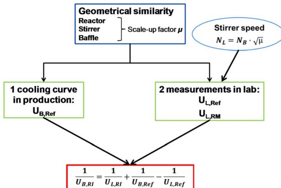
The applicability and accuracy of this procedure was evaluated by comparing 4 different liquids, i.e. solvents (Butylene glycol, Fabrication oil, Isoparaffine, Mineral oil) with water as reference liquid in the temperature range between 40°C and 90°C. The calorimetric laboratory measurements were done with the Mettler-Toledo RC1 in a 1.5 ltr. steel reactor. The plant reactor was a 13 m<sup>3</sup> glass lined reactor with double jacket and oblique blade agitator.
