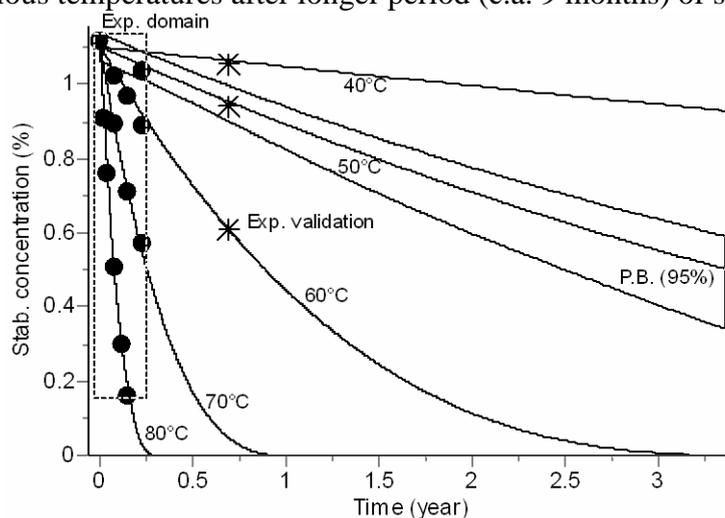
Fig.1 Prediction of change of stabilizer concentration in double base propellant based on the data collected in experimental domain depicted on the plot. Prediction curves at 40, 50 and 60°C were verified by the experimental points marked by asterisks. The prediction band PB is shown for the simulations of the process course at 50°C.
