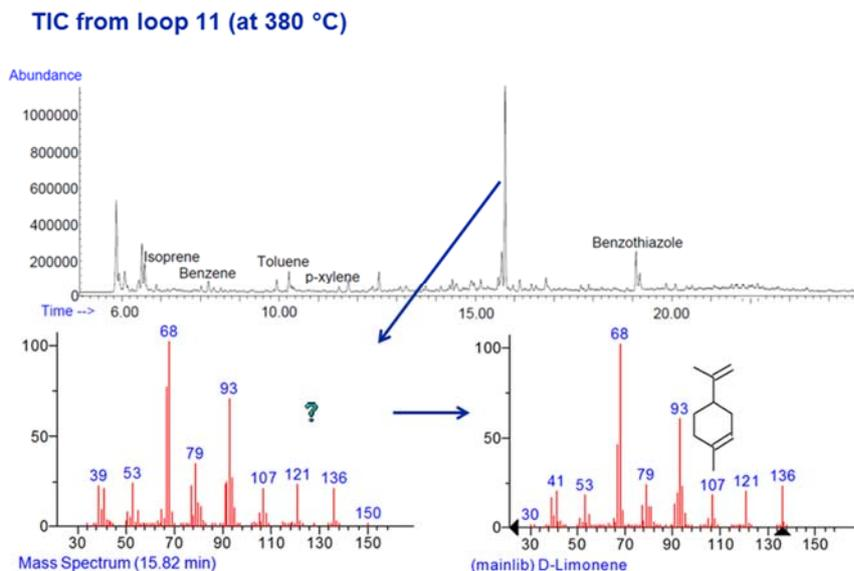
Figure 1: Total ion chromatogram (TIC) for loop 11, the MS at 15.82 min and its identification as D-Limonene.
