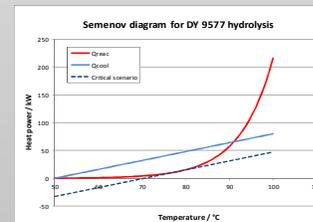
Semenov diagram for determination of critical jacket T
