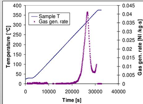
Gas release at constant volume (autoclave)
