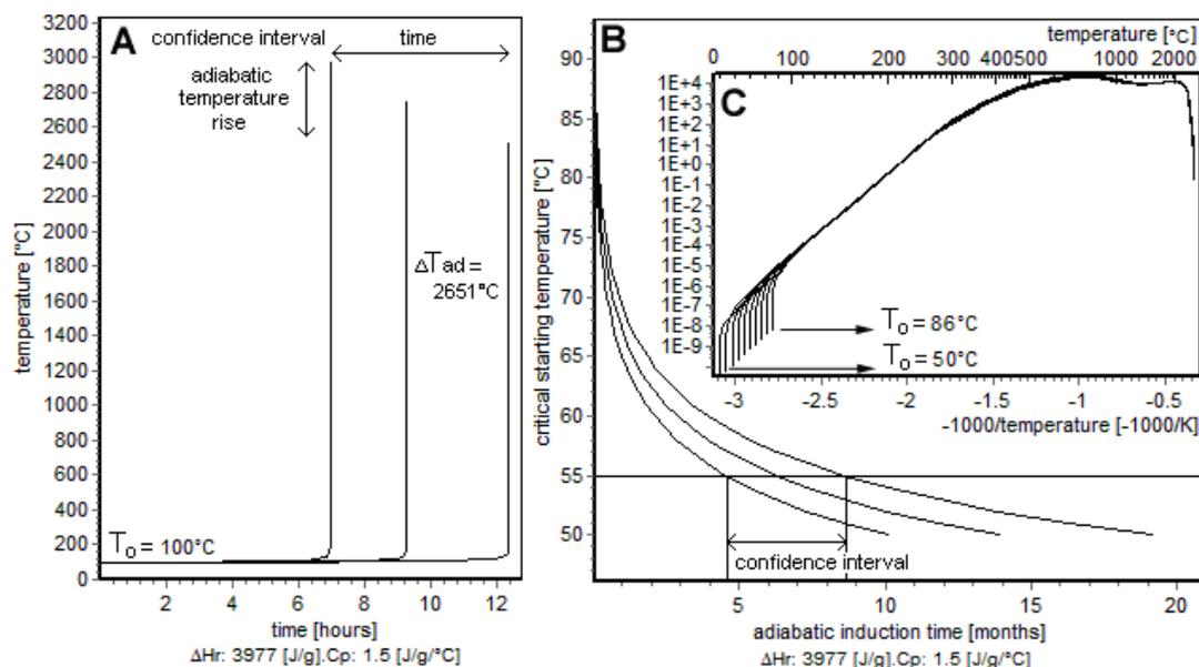
**Fig. 1** (A) Adiabatic runaway curves for a boost propellant (isochoric conditions) showing the confidence interval for the prediction ( $T_{\text{begin}}=100^{\circ}\text{C}$  and  $\Delta T_{\text{ad}}=\Delta H_r/c_p=2651\pm 233^{\circ}\text{C}$ ). The confidence interval was determined for 95% probability.
