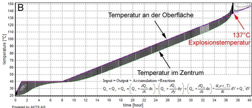
**Fig. 2** Slow cook-off experiments of a nitrocellulose based substance (A) and simulation (B). As presented in the figure, the predicted temperature of explosion was 137°C. It is in good agreement with the slow cook-off experiments (138°C).
