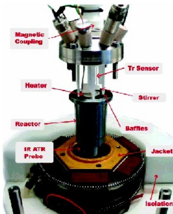
**Fig. 1** Latest version of the small-scale reaction calorimeter (sample volume 20 - 45 ml) with reactor jacketed made of copper and removable reactor (Hasteloy C22). The reactor is pressure resistant up to 20 bar, Temperature rage -20 ... 200 °C.<sup>6</sup>
