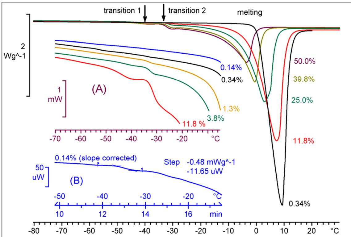
**Figure 1:** DSC curves (exo up) of different sucrose solutions measured at 5 K/min. The curves show two endothermic steps at around  $-44\text{ }^{\circ}\text{C}$  (transition 1) and  $-35\text{ }^{\circ}\text{C}$  (transition 2) and a melting peak. In diagram (A) the region of the transitions 1 and 2 are magnified for clarification. Diagram (B) shows a slope corrected curve of the solution with 0.14wt% sucrose.
