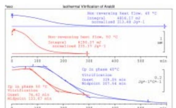
Fig. 7. Isothermal vitrification of Araldit. The non-reversing heat flow curve shows the course of the vitrification. The  $C_p$  in-phase curve shows how the specific heat decreases during the reaction.
