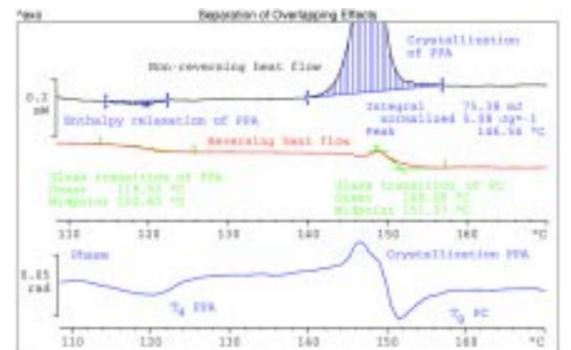
Fig. 4. ADSC of a mixture of Polyphthalamide (PPA) and Polycarbonate (PC). The non-reversing heat flow first shows a slight enthalpy relaxation during the glass transition and the crystallization of PPA. The glass transitions of PPA and PC are seen in the reversing curve and also, but less clearly, in the phase curve. In a conventional DSC measurement, the glass transition of the PC would be hidden by the crystallization peak of the PPA.
