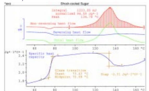
Fig. 5. ADSC of shock-cooled amorphous sugar. The glass transition can be seen in the reversing heat flow curve at about 75 °C. The non-reversing curve shows the crystallization. Both the glass transition and the crystallization can be clearly seen in the specific heat capacity curve.
