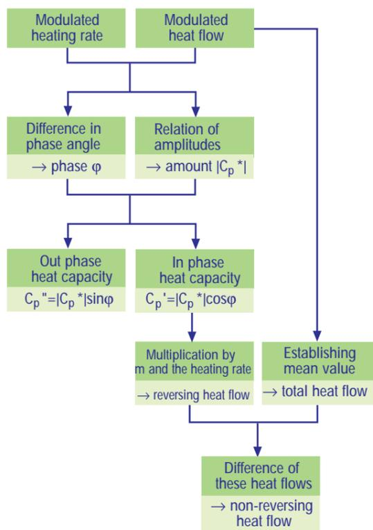
Fig. 2. Evaluation and results of a modulated DSC curve
