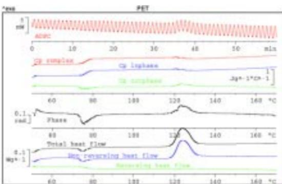
Fig. 3. ADSC evaluation of PET. The glass transition can be seen in the reversing heat flow curve, and the enthalpy relaxation and the cold crystallization in the non-reversing heat flow curve. The total is equivalent to a non-modulated DSC curve. A typical indication of the glass transition is the negative peak shown by the phase curve at about 75 °C.
