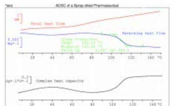
Fig. 6. ADSC of a spray-dried pharmaceutical formulation with a residual moisture content of 10.8%. Both the reversing heat flow and the complex heat capacity curves clearly show the glass transition at about 110 °C. This cannot be seen in the total heat flow curve because of the evaporation of the water.
