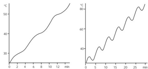
Fig. 1. Temperature programs with various parameter settings: left,  $\beta_0 = 2$  K/min,  $A_T = 1$  K,  $P = 5$  min, right,  $\beta_0 = 2$  K/min,  $A_T = 3$  K,  $P = 5$  min
